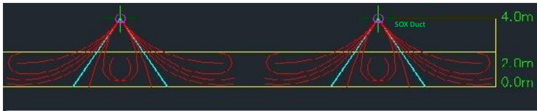
Airflow Distribution of DurkeeSox Air Dispersion System
